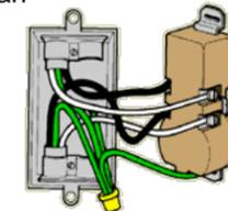
**30** **NEC 200.7** Where permanently re-identified at each location where it is visible and accessible, the conductor with white colored insulation in type NM cable may be used as an ungrounded conductor. The re-identified conductor shall not be used as the return conductor from a switch to an outlet.
